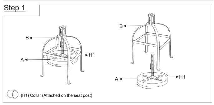
Remove Seat (A) from its shipping position by disengaging seat post from the top of Base (B) assembly. Remove Collar (H1) from the seat post. Remove Seat (A) and turn upright as shown in the following step.
